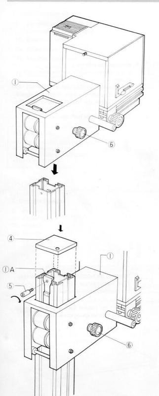
Loosen the carriage lock knob (6) by turning it counter-clockwise. Lift the entire head assembly as shown, matching the column and the opening of the carriage, and put the assembly over the column.
