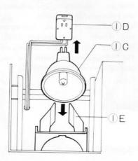
Pull the lamp socket (1D) out of the chamber. Put the enlarging-lamp (1C) in the socket, and put the lamp in the lamp-holder frame (1E) inside the chamber as shown.
