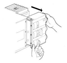
Let the module slide forward as shown, off the lamphouse.
